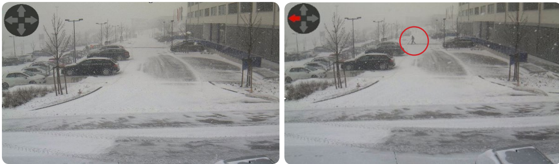
The snowfall here will not trigger a movement alarm; yet, the person moving from right to left in the background will be detected.
